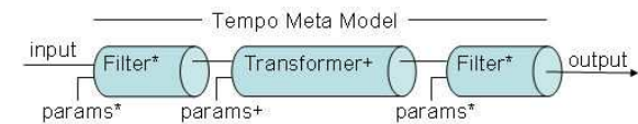
Figure 3. The Tempo pipeline meta model where “*” means zero or more and “+” one or more.
