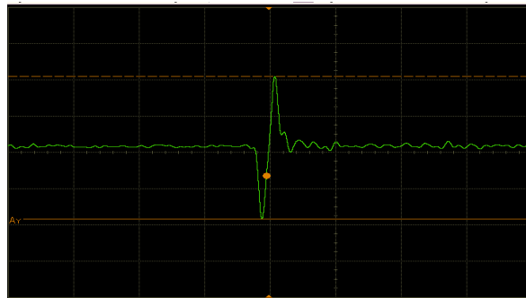
Fig. 6. Output waveform of the proposed radar transmitter
