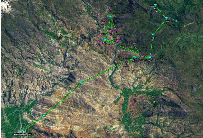
**Fig.3.** Final network design seen through Radio Mobile software
